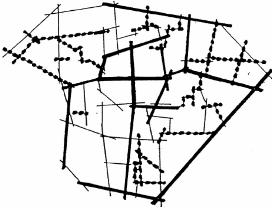
Figure 5.7 Axial map of Apt with the 10% integration core shown in heavy black, and the 50% most segregated lines shown dotted
